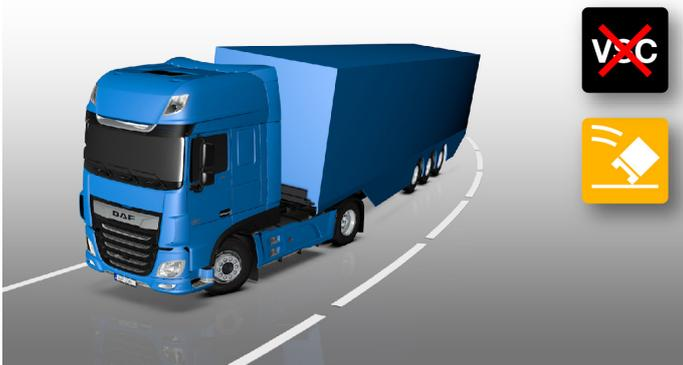
In case of understeer the front of the vehicle slides to the outside edge of the curve and if uncorrected, will leave the road. VSC will apply the brakes at the curve-inside wheels to bring the tractor back on its intended path.
